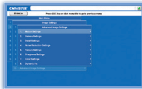
Virtual On Screen Display (OSD): access full menu structure, remotely.
